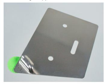
Used for service work at STAMA: high-precision Laminum HP2 laminated shims from MARTIN with 20 sheet metal films with a thickness of 0.05 mm and 5 with a thickness of 0.01 mm
