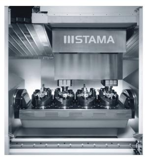
Multiple clamping system on bridge support: the STAMA MC 536 TWIN spindle milling machine in the 5-axis processing of wheel mounts. The spindle spacing here is 600 mm.
